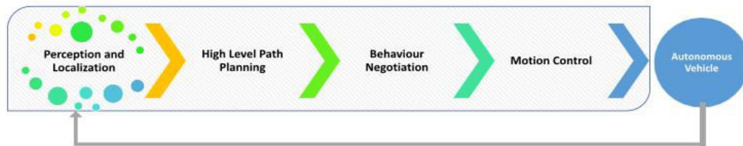
Figure 1. Architecture of a perception, planning, and control workflow in autonomous vehicles
