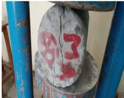
Fig 4.2 split tensile Strength test
