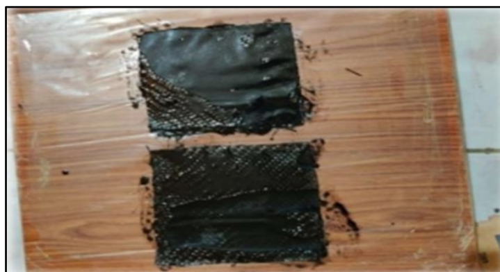
Figure 2: Samples Prepared by Using Hand Layup Process
