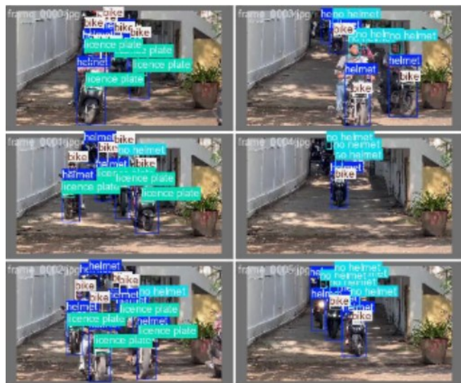
Figure 2: Real-time video frame showing bounding box detection for person, motorcycle, and number plate with successful OCR extraction
