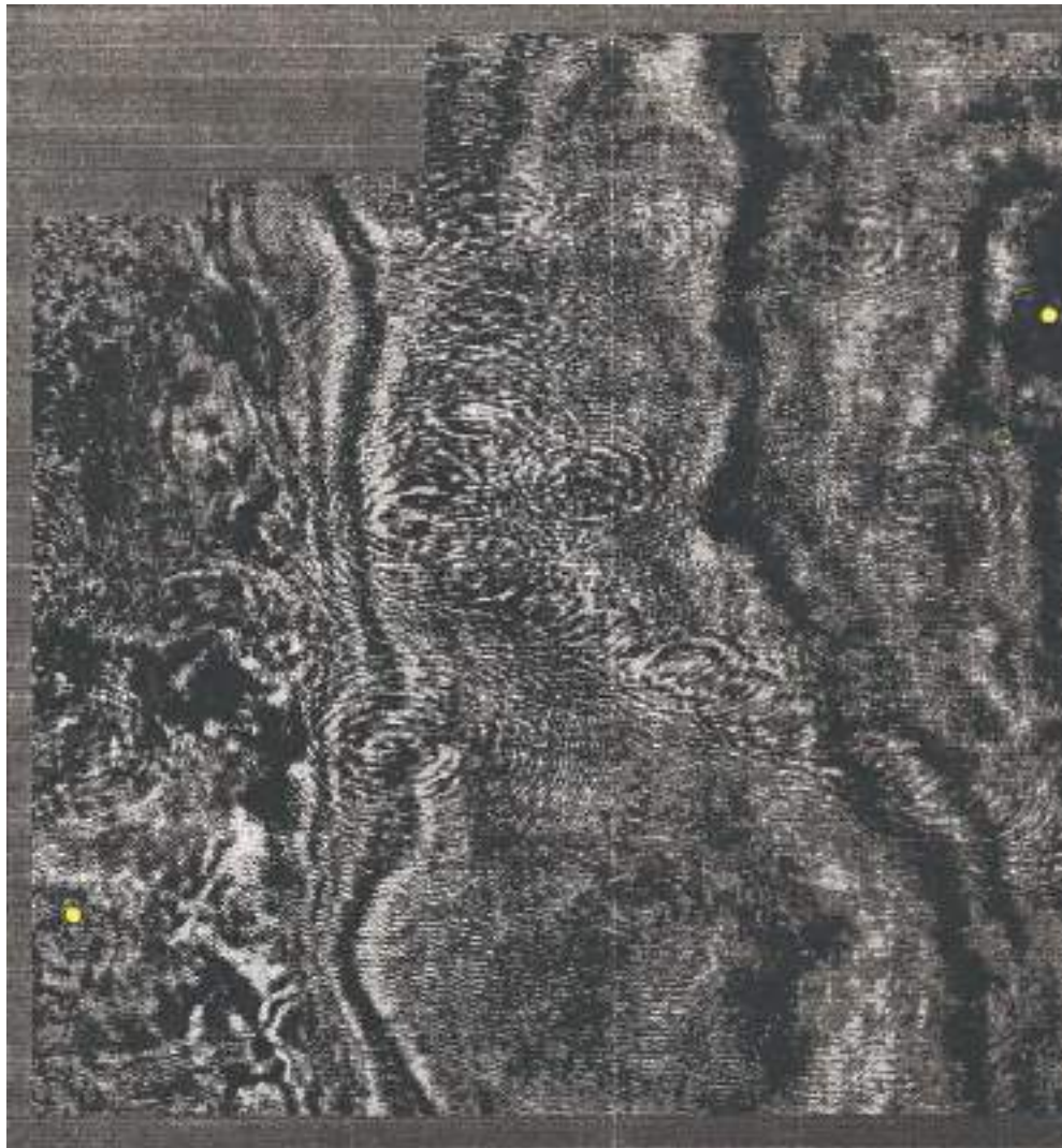
Figure (5): presents a time slice extracted from an unmigrated 3-D stacked data volume, displaying circular features that are linked to point scatterers located along sea-bottom pipelines. (Data provided by Total Argentina; adapted from Yilmaz, 2001).
