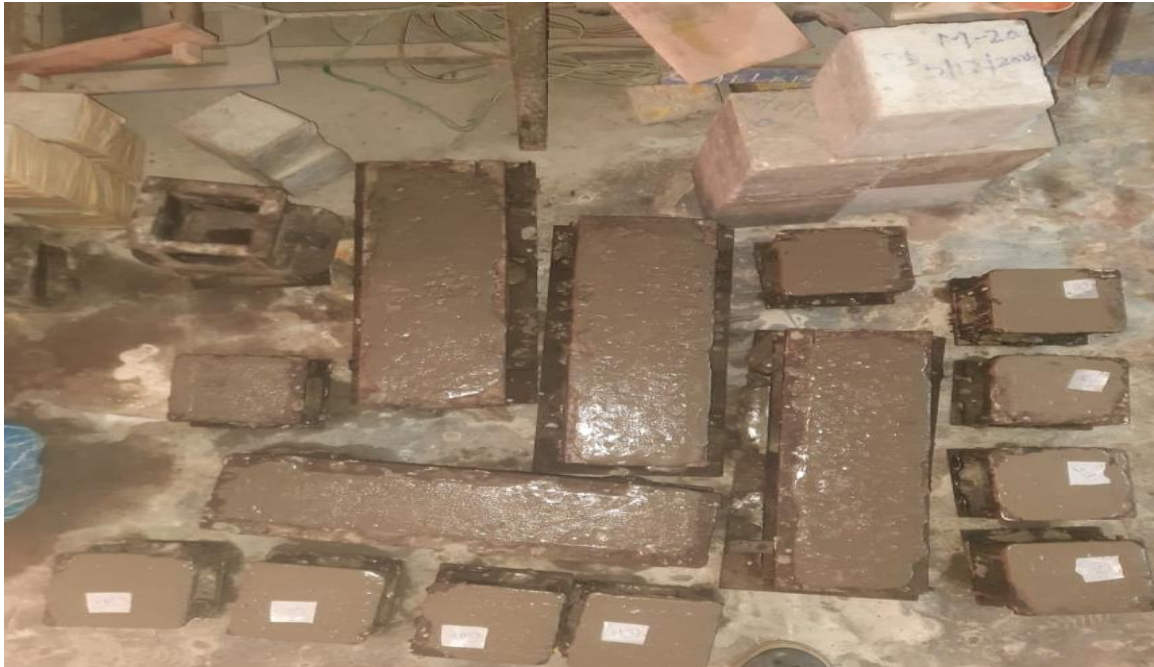
Figure 2 Casting of Cubes
